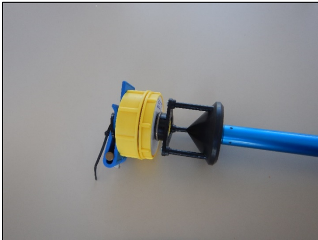
Figure 3. To measure trees within a 360° circle, the transponder is attached to the 360° cone which itself is fastened to the top of the plot center staff.
