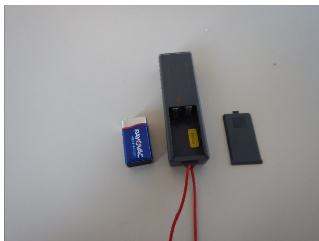
Figure 5. The distance-measuring unit will take a 9V battery inserted into the battery casing at the bottom of the unit.
