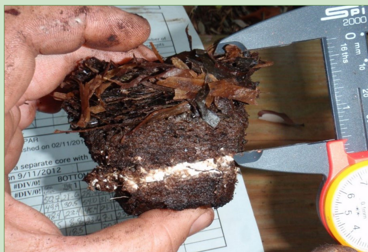
Figure 2. Measuring accretion, which is the material deposited above the white line. The white line is feldspar, a mark layer placed at the site on a previous sampling event. Here we can see turtle grass ( Thalassia testudinum ) that is becoming incorporated into the soil.
