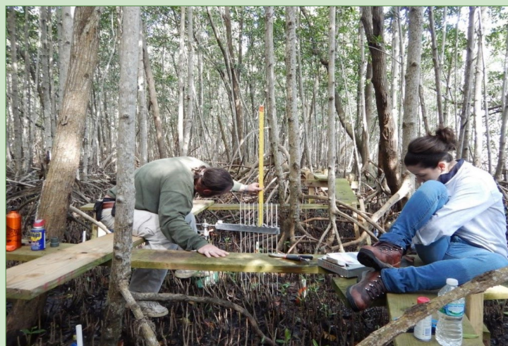
Figure 1. Kevin Whelan, SFCN ecologist, is measuring soil surface elevation using the Soil Elevation Table (SET). The SET is attached to a permanent benchmark. The height of the pins transcribes the elevation of the soil and standardizes it to a fixed reference point (the metal arm). Repeated measurements over time monitor the rate of soil elevation change.
