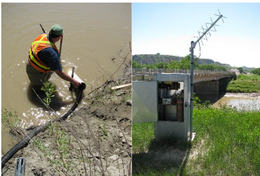
Figure 3. A sonde device is used to measure water quality in the Little Missouri River at Theodore Roosevelt National Park (right panel). The United States Geological Survey Little Missouri gaging station (06336000) is set up for real-time data transmission via satellite (left panel). Photographs courtesy of NPS.
