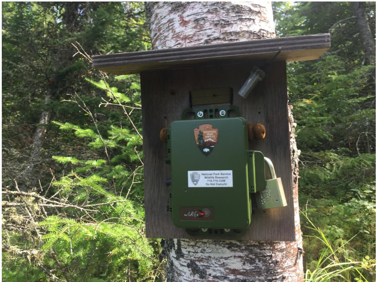
Figure 2. Example of automated recording device (ARS) deployed in the field. This device is attached to a backer board with a strap around the tree. The temperature logger is attached under the roof of the backer board ( upper right ).
