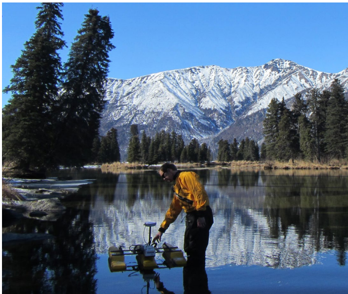
Preparing the Acoustic Doppler Current Profiler for a discharge measurement at the outlet of Kijik Lake in Lake Clark National Park and Preserve.
