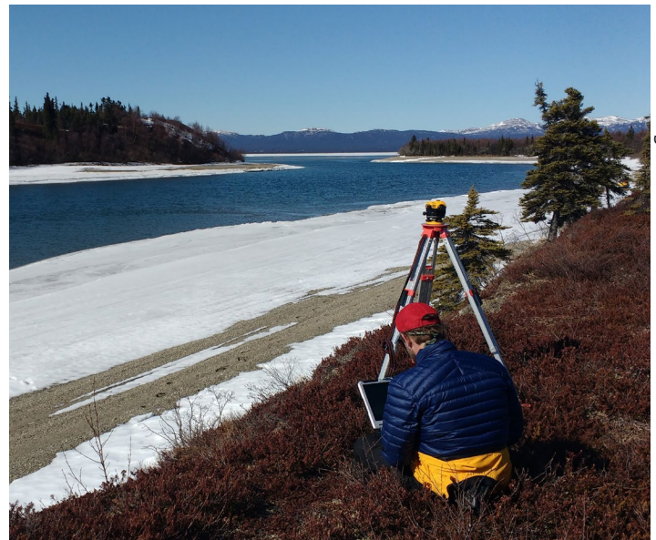
Using a transit level and field computer to survey and record level logger elevation at the outlet of Lake Clark in Lake Clark National Park and Preserve.
