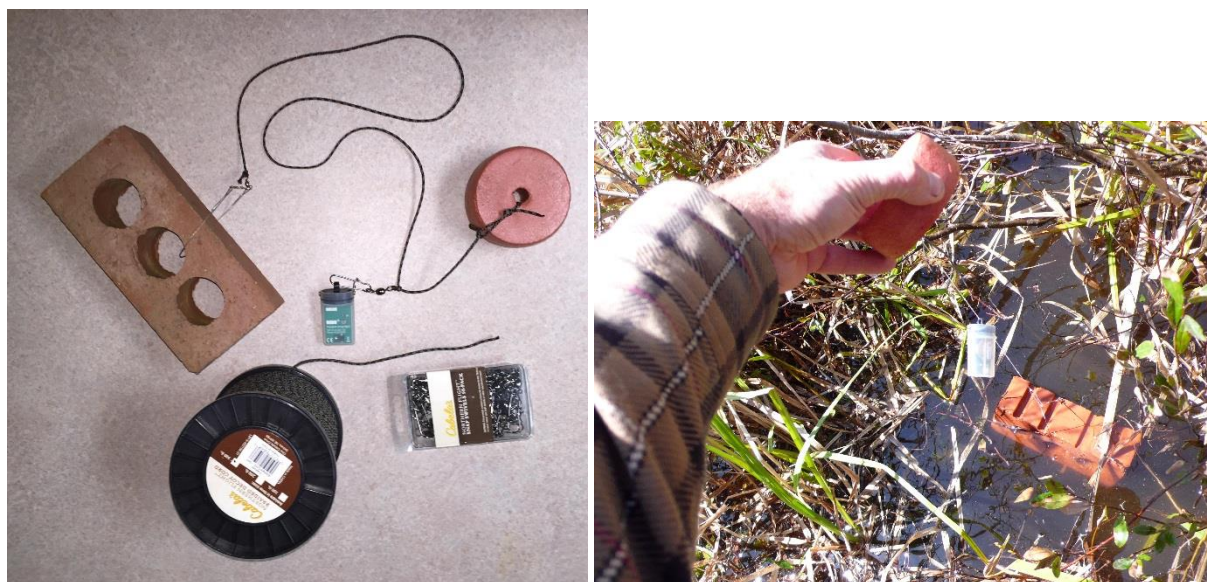
Figure 8. Example materials for temperature logger placement using a weight ( left ), and field application ( right ).
