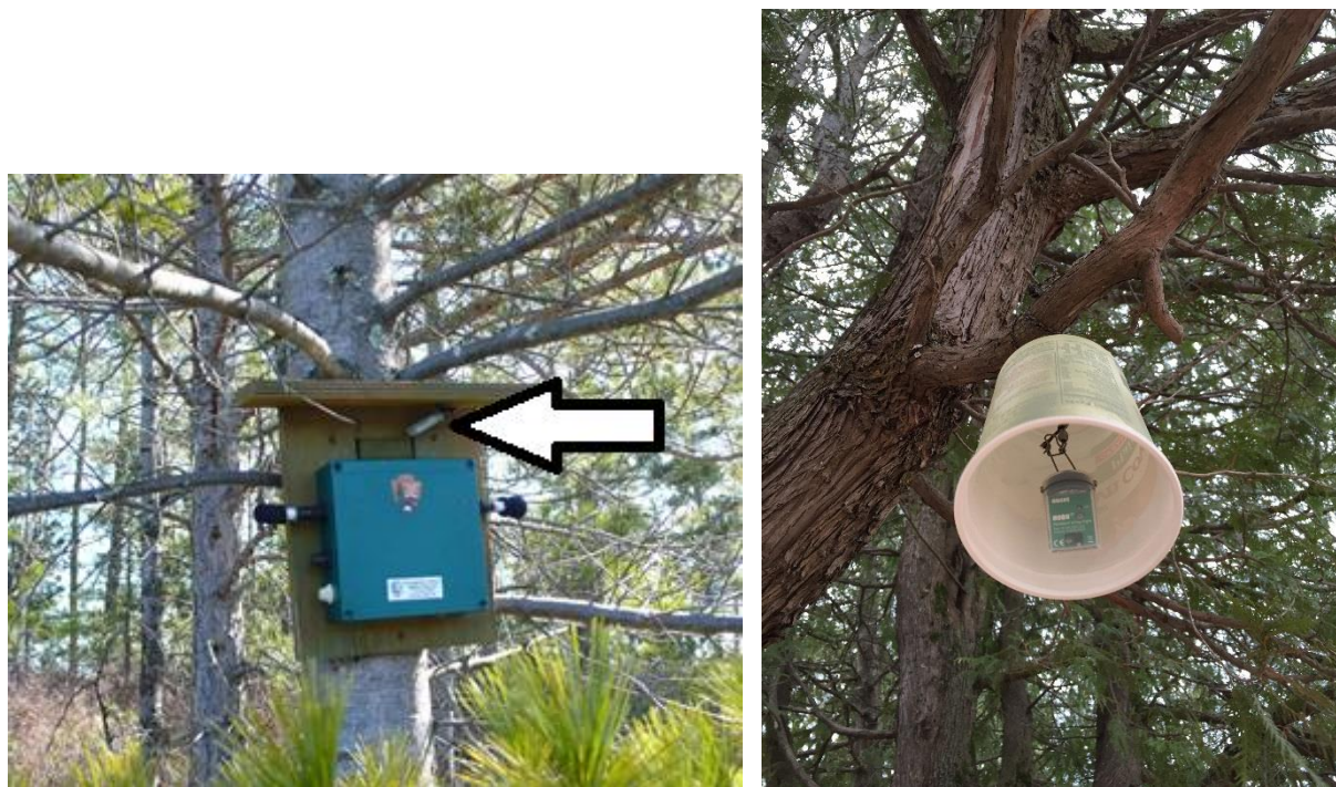
Figure 7. Temperature logger mounted under roof of backer board ( left ), or in cup for solar shielding ( right ).
