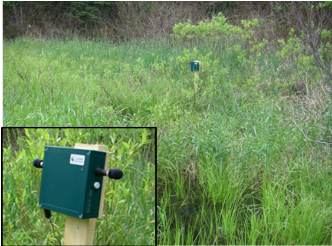
Figure 2. Song Meter mounted to a 2×4 stake pounded in the ground. This 2×4 could be painted to blend with the environment better and will have to be replaced every 2–4 years. Consider a 4×4 cedar post for longevity.
