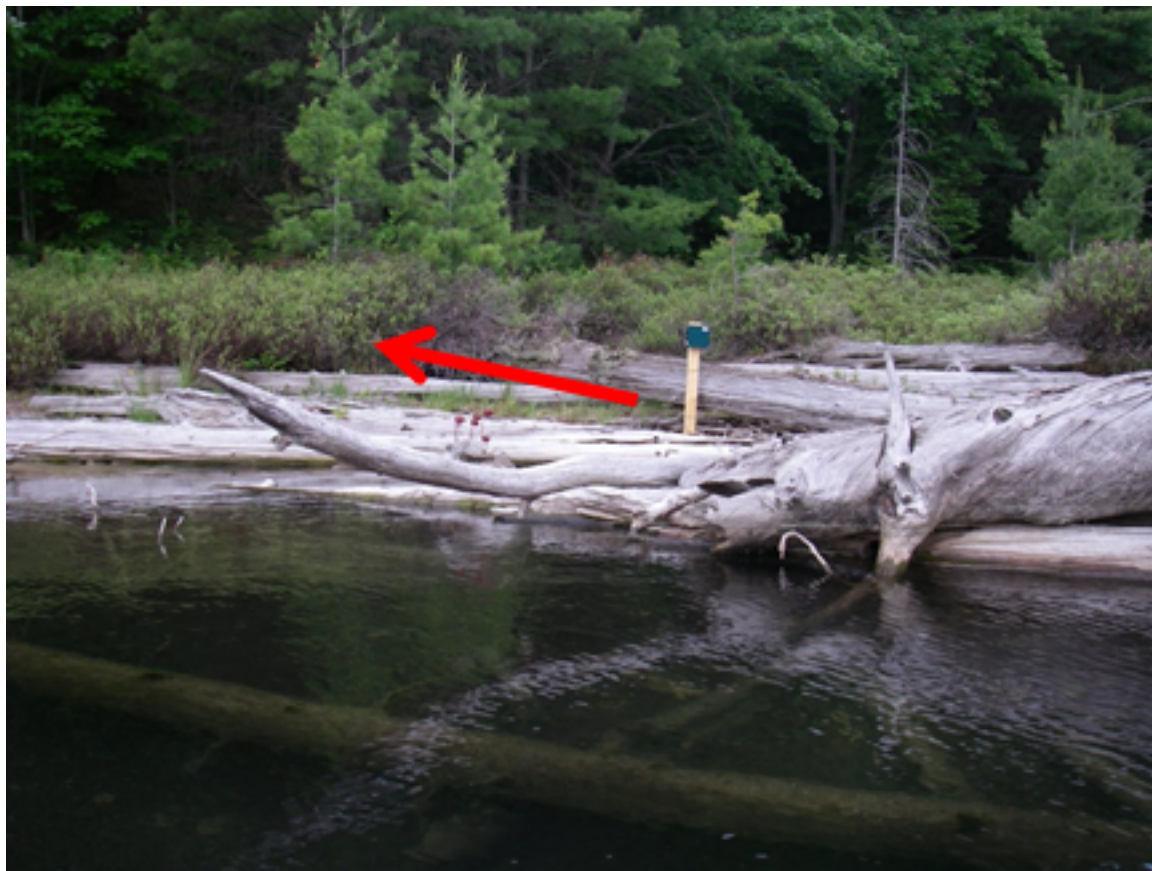
Figure 3. Song Meter could be moved back and closer to background vegetation onto the historical high-water mark ( arrow ) to blend in better and save from being inundated in wet years.
