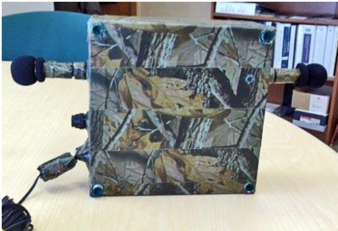
Figure 4. Camouflage tape can be used reduce people finding and tampering with the Song Meters.
