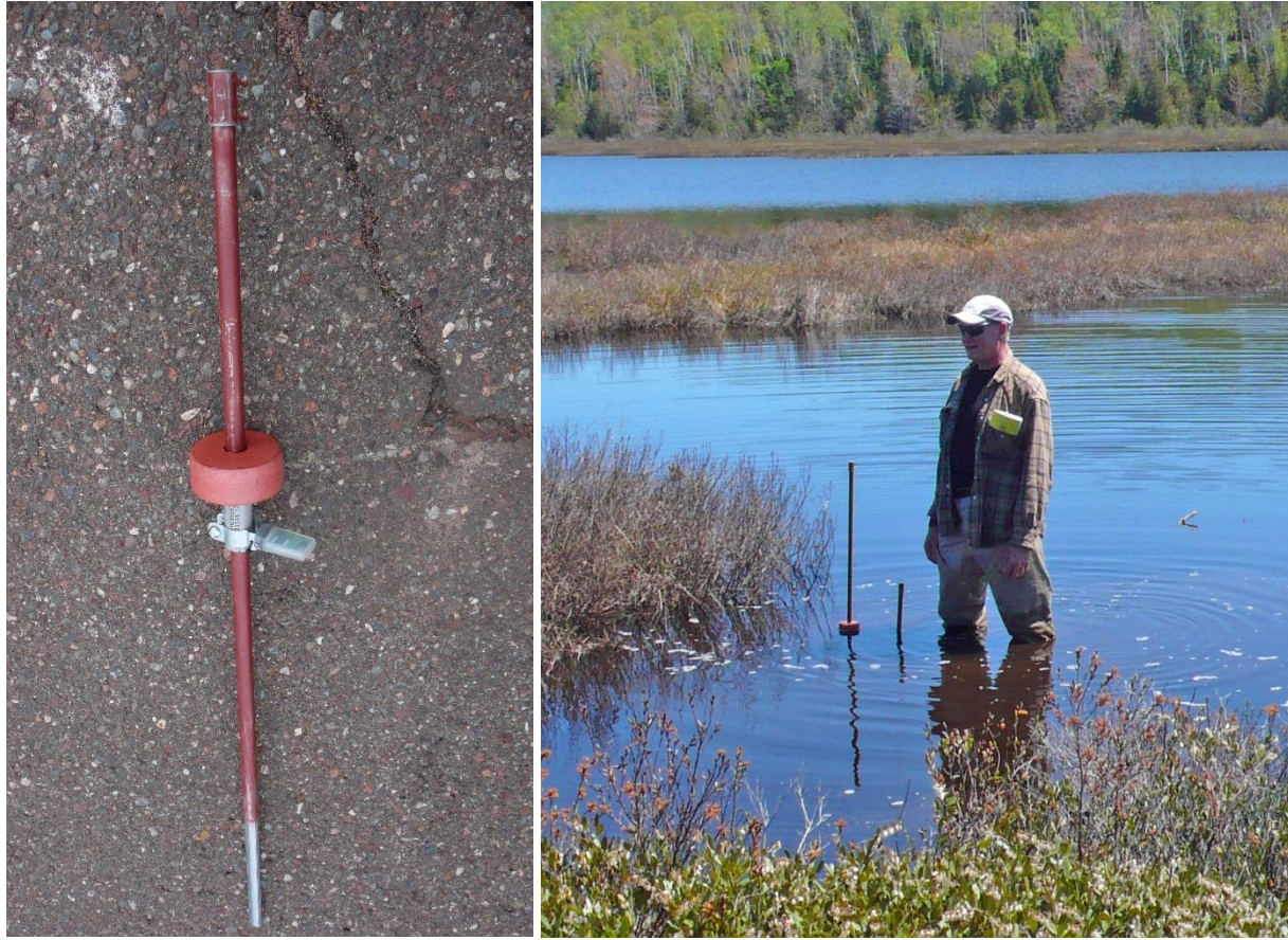
Figure 9. Mounting temperature logger option for recording near water surface temperature ( left ), and field application ( right ).
