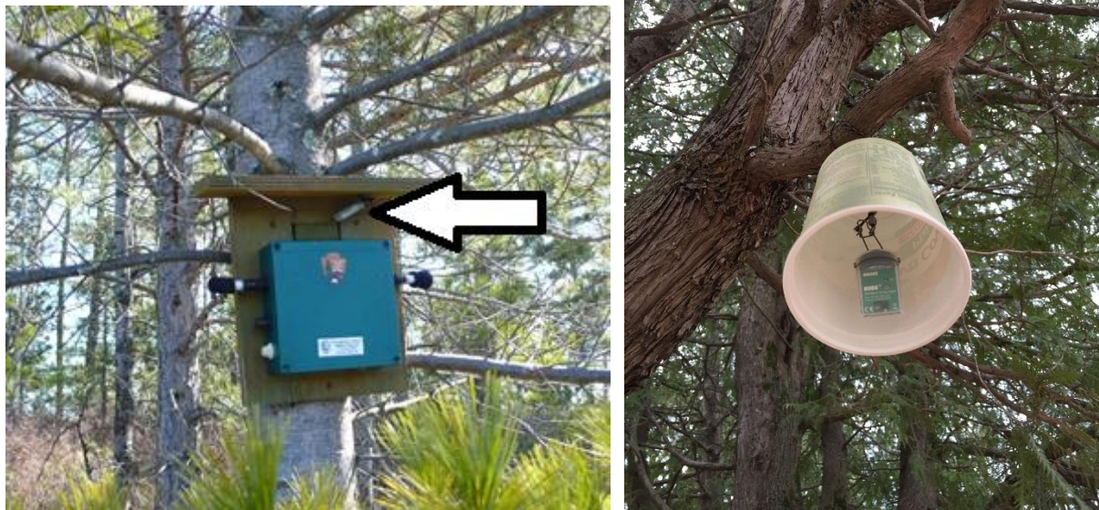
Figure 9. Temperature logger mounted under roof of backer board ( left ), or in cup for solar shielding ( right ).
