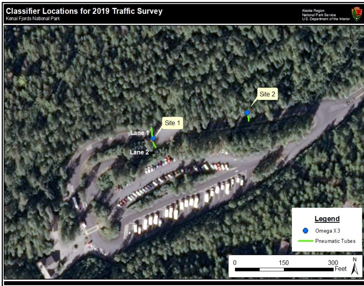
Figure 1. Locations of the Omega X3 vehicle classifier and pneumatic road tubes at Site 1 and Site 2.
