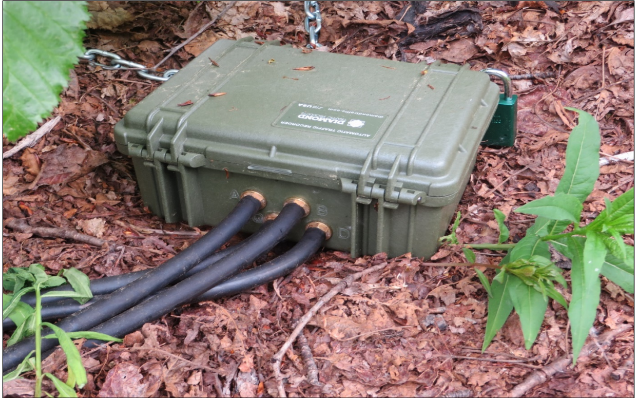
Diamond Omega X3 vehicle classifier with four road tubes connected (NPS/Tyler Balstad).
