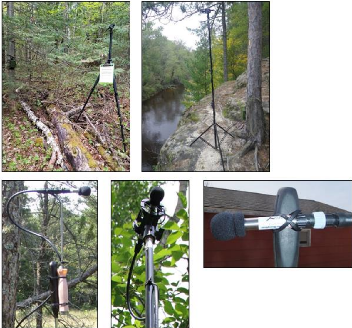
Figure 1. Examples of equipment set up using the tripod to hold the microphone and a nearby tree to hold the Song Meter. NPS PHOTOS.
