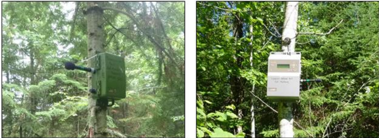
Figure 4. Examples of equipment mounted on a tree trunk with microphone directly attached to Song Meter. NPS PHOTOS.
