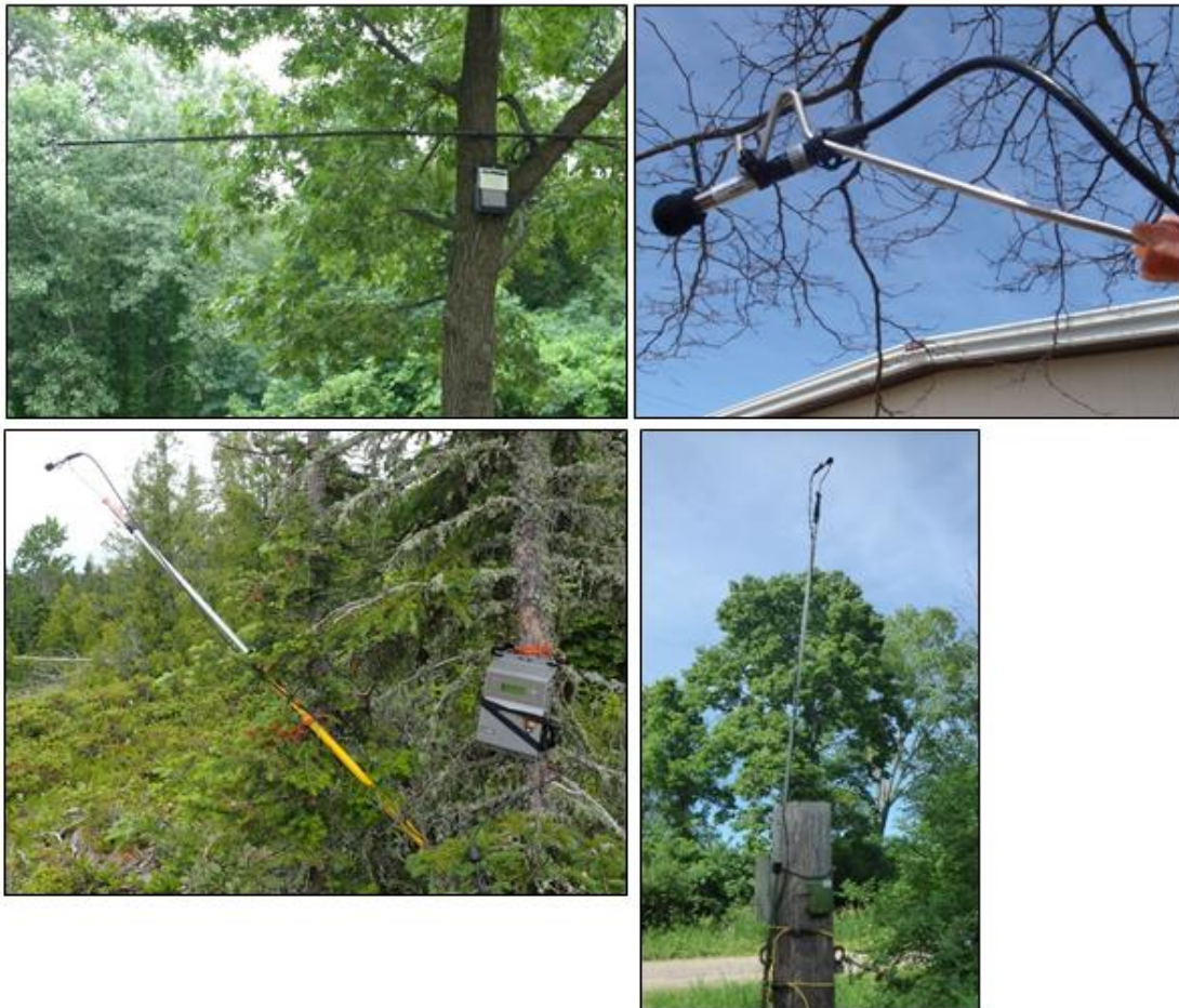
Figure 3. Examples of equipment set up using a telescoping painter's pole. NPS PHOTOS.
