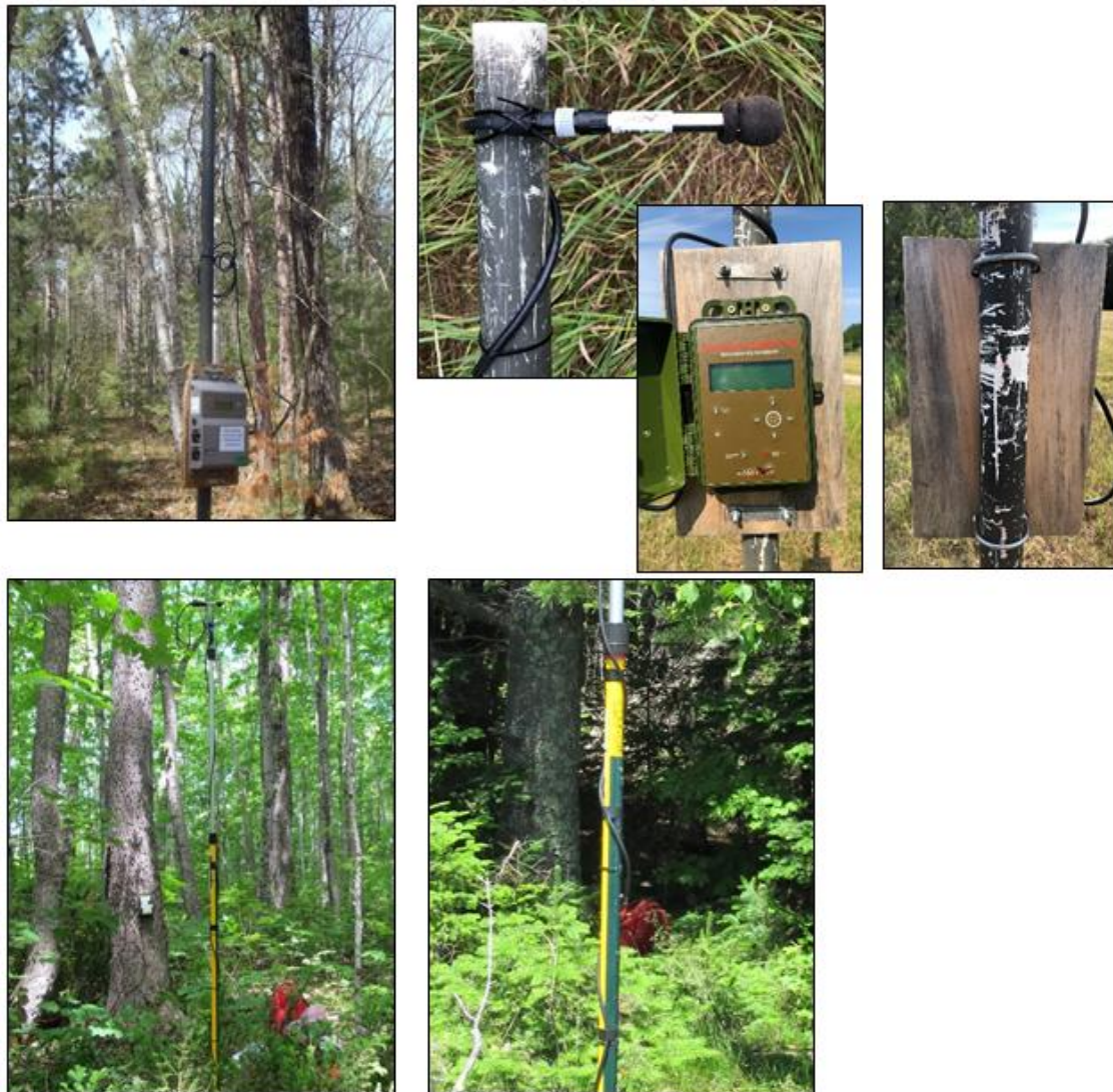
Figure 2. Examples of equipment set up using a T-post with PVC ( top ) and T-post with painter pole ( bottom ). Inset photos demonstrate attachment of the Song Meter to a backing board and the backing board to the post using U-bolts. NPS PHOTOS.
