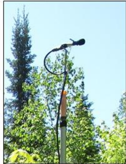
Figure 5. Loops should be created in microphone cables. Rainwater will drip off the bottom of the loop, rather than flowing into the microphone port or microphone base.
