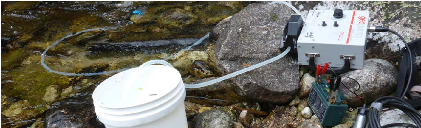
Collection of an eDNA sample from a stream. On-site filtration using peristaltic pumps is a common method (note the blue filter unit visible at the end of the intake tubing in the upper left).
