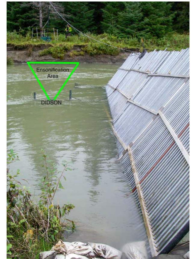
Figure 2. The Bartlett River DIDSON site displaying the DIDSON attached to the H-mount, upstream of the partial weir. The green electronics box containing batteries, fuel cell, computer, hard drives and DIDSON switch box is located in the center background.
