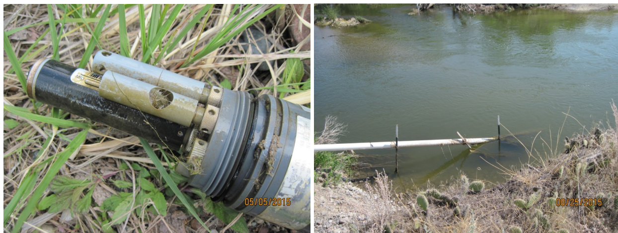
Figure 4. A sonde device is used to measure water quality in the Laramie River at Fort Laramie National Historic Site. The United States Geological Survey Laramie River gaging station (06670500) is set up for real-time data transmission via satellite. Photographs courtesy of NPS.
