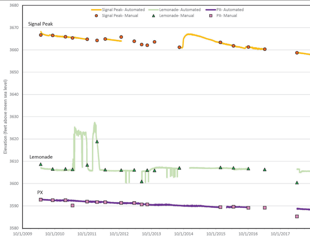
Figure 3-4. Water level elevation at three groundwater monitoring wells, water years 2010–2018, Guadalupe Mountains NP
