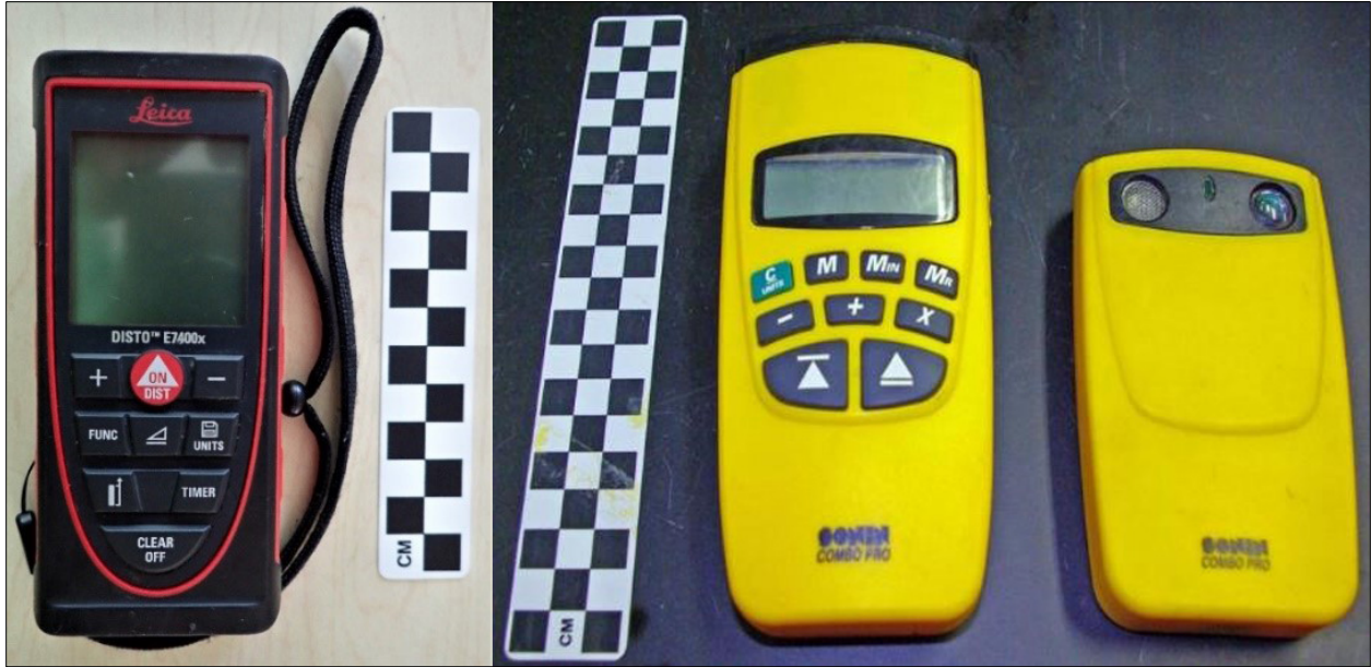
Figure 8. Rangefinders used to determine cluster distance from the baseline. The Leica Disto™ E7400x (left image) is a self-contained rangefinder. The Sonin Combo Pro™ (right image) rangefinder includes a transmitter (left) and a receiver (right).
