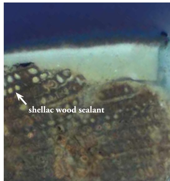
Figure 172: Ultraviolet Light 100x- SPI05. The substrate of the sample appears to have shellac embedded in the wood pore structure. Shellac was a commonly used sealer applied to new wood prior to the application of paint.
