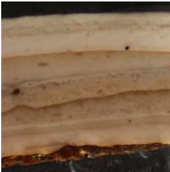
Figure 160: Visible Light 200x- SPI01. Based on the paint cross-sections examined, the diamond on the apron was installed at the same time as the mantel. The initial pigmented transparent finish is seen in both sample SPI01 and SPI02.
