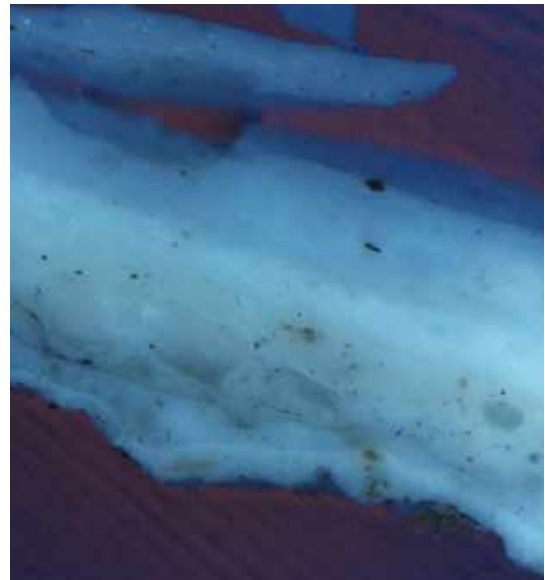
Figure 169: Ultraviolet Light 100x- SPI03. Note bluish autofluorescence which is characteristic of limewash coatings.
