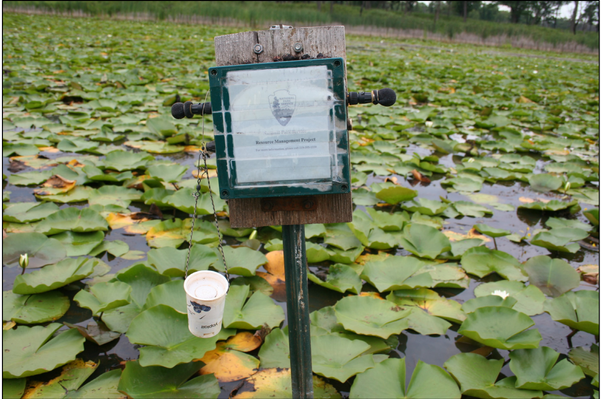
Figure 2. Example of automated recording device (ARS) deployed in the field. This device is attached to a backer board and to a metal t-post. The temperature logger is located in a shaded cup. With new SM4 units replacing old SM2+ units (shown here) in 2019, we recommend a roof be added to the backboard to better protect the ARS from rain, sun and birds, and that the logger be hung in the shade either under the roof or in a nearby shrub or tree.
