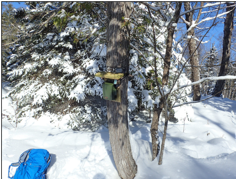
Figure 2. An automated recording device deployed in the field. This device is attached to a backer board and strapped to a tree trunk. The temperature logger is located under the backboard roof.
