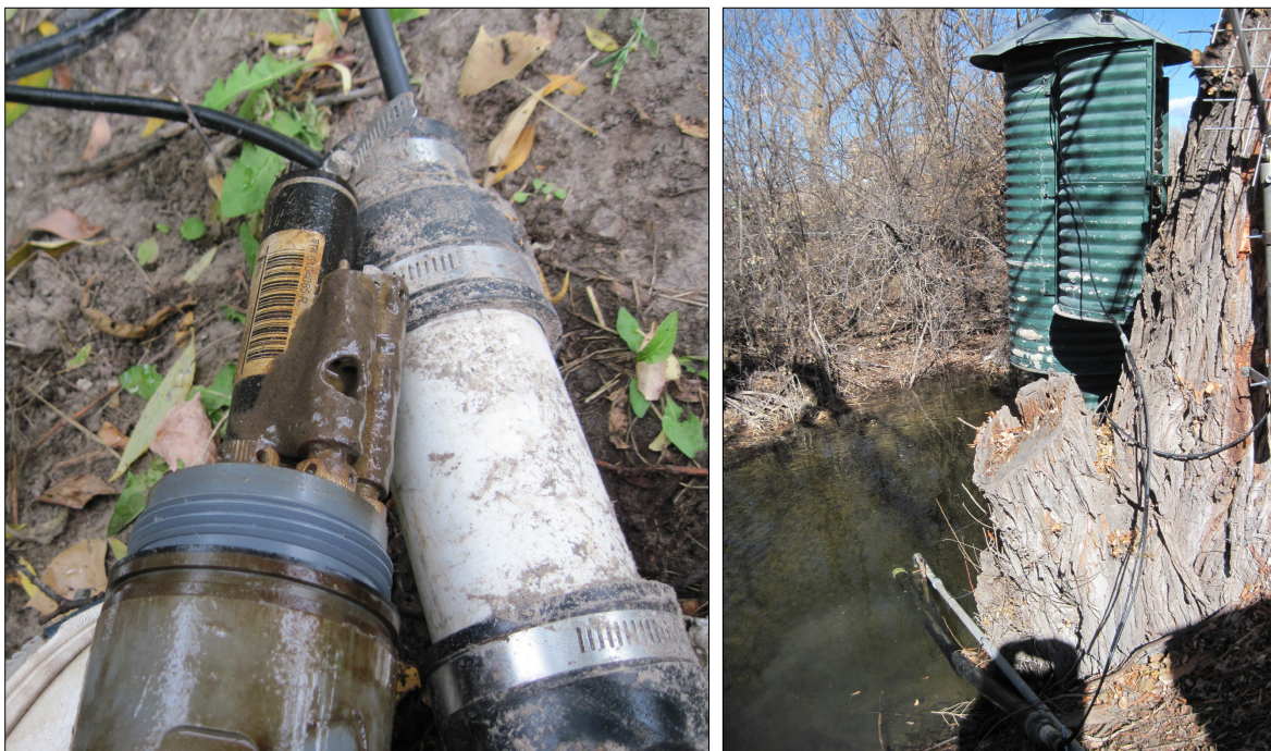
Figure 3. A sonde device is used to measure water quality in the Niobrara River at Agate Fossil Beds National Monument. The United States Geological Survey Niobrara River gaging station (06454100) is set up for real-time data transmission via satellite. Photographs courtesy of NPS.
