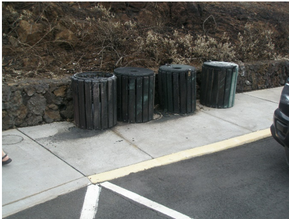
Photo 3. Fire-damaged waste disposal bins.
