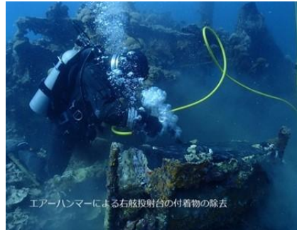
2. Coral cleaning with an air hammer drill
