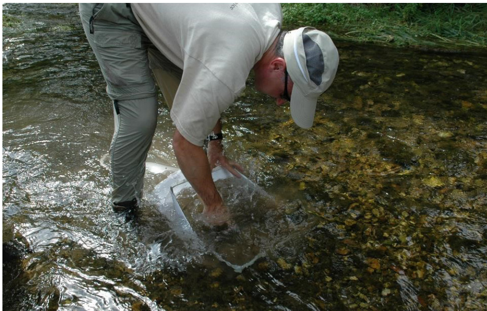
Collecting invertebrates with a Surber sampler. NPS.
