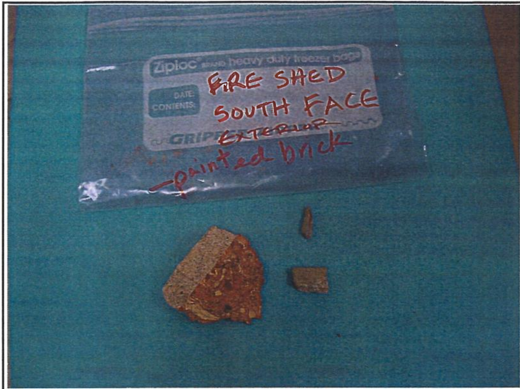
Photo 16. Fire Protection Shed – Mortar/brick samples from south face. Brick painted on side not shown.
