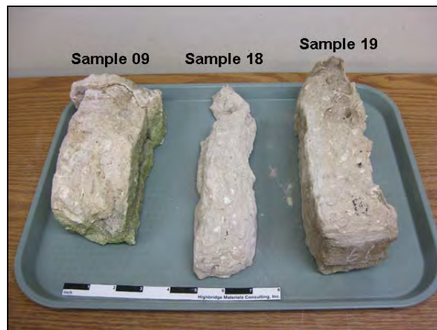
Figure 1: Photographs of the three tabby brick samples used for the qualitative salt determination through x-ray diffraction analysis.
