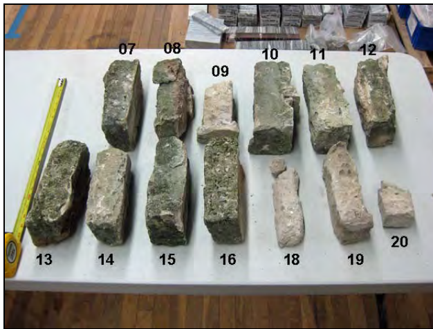
Figure 1: (Left) Photograph of the tabby brick samples provided to Highbridge for various testing. Sample 07 was used for this compositional analysis. Samples 09, 13, and 19 was used for supplemental information. (Right) The client also provided a sample of the local sediment. This was compared to the sands extracted from the brick units.
