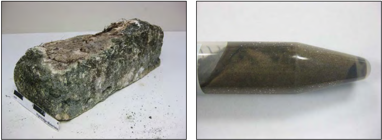
Figure 1: (Left) Photograph the tabby brick sample used to extract a clay sample. Sample 07 was used for this purpose. (Right) Photograph of the clays extracted from Sample 07. The extracted material is shown in the centrifuge tube.
