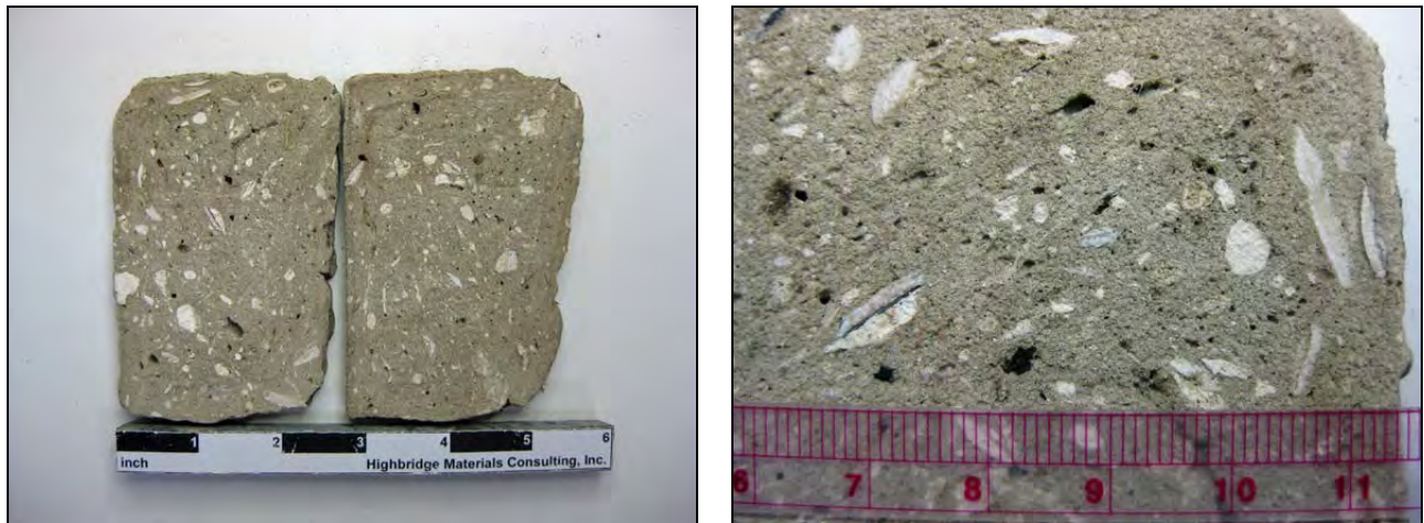
Figure 3: The texture of the tabby brick is shown in these images of sawn and ground cross sections. The right image is a close-up with a scale bar having units in centimeters. The matrix is a pale brown color likely due to the inclusion of trace organic impurities in the sand. Unscreened fragments of partly burned shell are evenly dispersed throughout the brick without producing a grain anisotropy.
