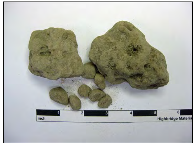
Figure 1: (Left) Photograph of the tabby brick samples provided to Highbridge for various testing. Sample 07 was used for this compositional analysis. Samples 09, 13, and 19 was used for supplemental information. (Right) The client also provided a sample of the local sediment. This was compared to the sands extracted from the brick units.
