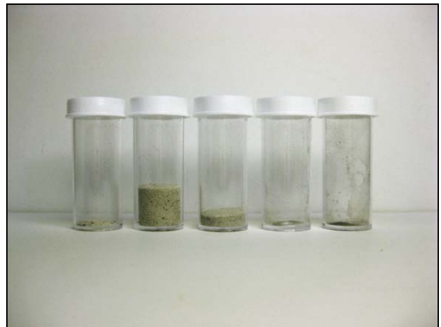
Figure 2: Photographs of the aggregate extracted through acid digestion. The total extraction is shown at left. The sand is uniform and light yellowish-gray in color. At right, the sand is shown after grading through a standard sieve stack. The sand is very fine and somewhat narrowly graded.
