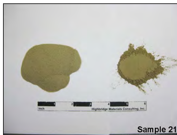
Figure 4: Photographs of the aggregate are shown after being extracted through acid digestion. In each image, the sand is shown to the left, and the silt and clay to the right. It is suspected that the latter also contains some organic matter. Note that the sand colors vary slightly while the color of the fines is somewhat consistent. Sample 21 represents the local sediment collected by the client. The fines content is much higher in this sample and the color does not differ from that of the sand.
