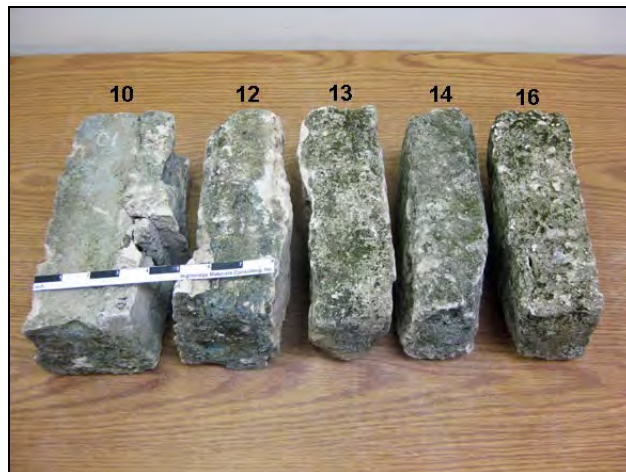
Figure 1: Photographs of the tabby brick units from which compressive strength and absorption test specimens were prepared.
