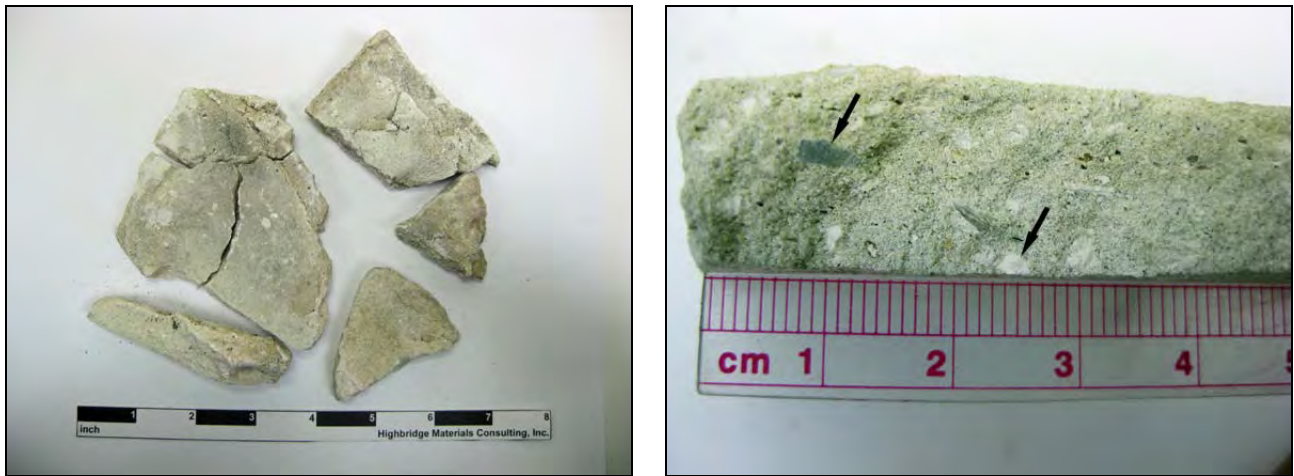
Figure 1: Photographs of the mortar sample received by Highbridge for examination. The total sample is shown at left. A fractured surface is shown at right. The arrows illustrate undispersed lime grains and incompletely burned shell fragments.
