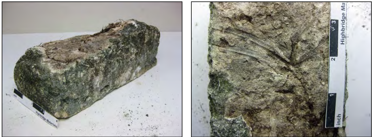
Figure 2: Photographs of Sample 07 used by the laboratory for the compositional analysis of the tabby brick. The whole brick is shown obliquely in the left image. A close-up of one bed surface is shown at right. There is an unusual set of tool marks on this surface
