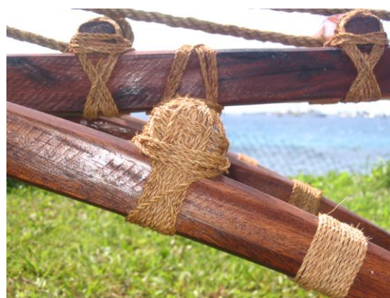
Ino in lejrōñ (unique square lashing) on the kein ioon ere. Notice all lashing line are Ekkwal or coconut sennit.
