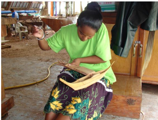
Trainee is lashing the keion ere or outrigger complex
