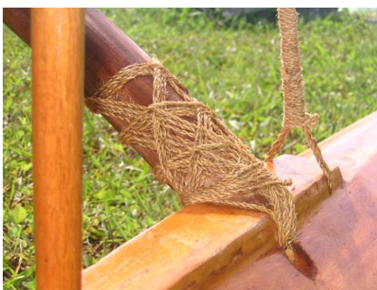
Lashing of the Apet or the secondary outrigger boom to the outrigger float.
