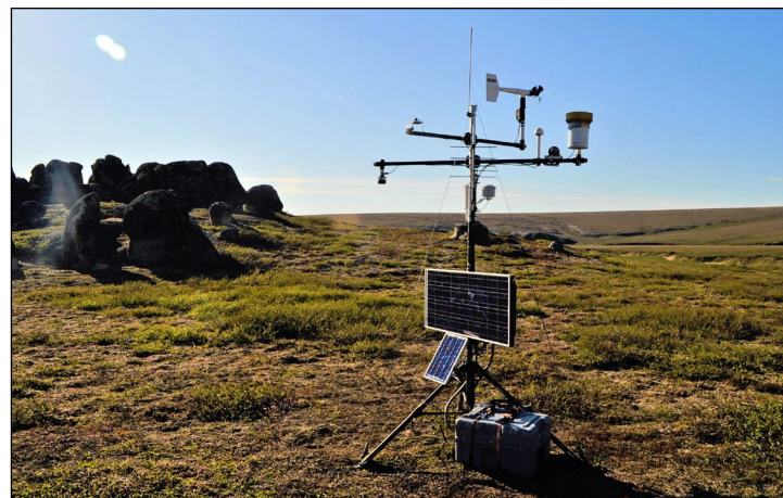
Figure 6. Serpentine climate station rain gauge (top right cylinder) records summer rainfall when temperatures are above freezing.
