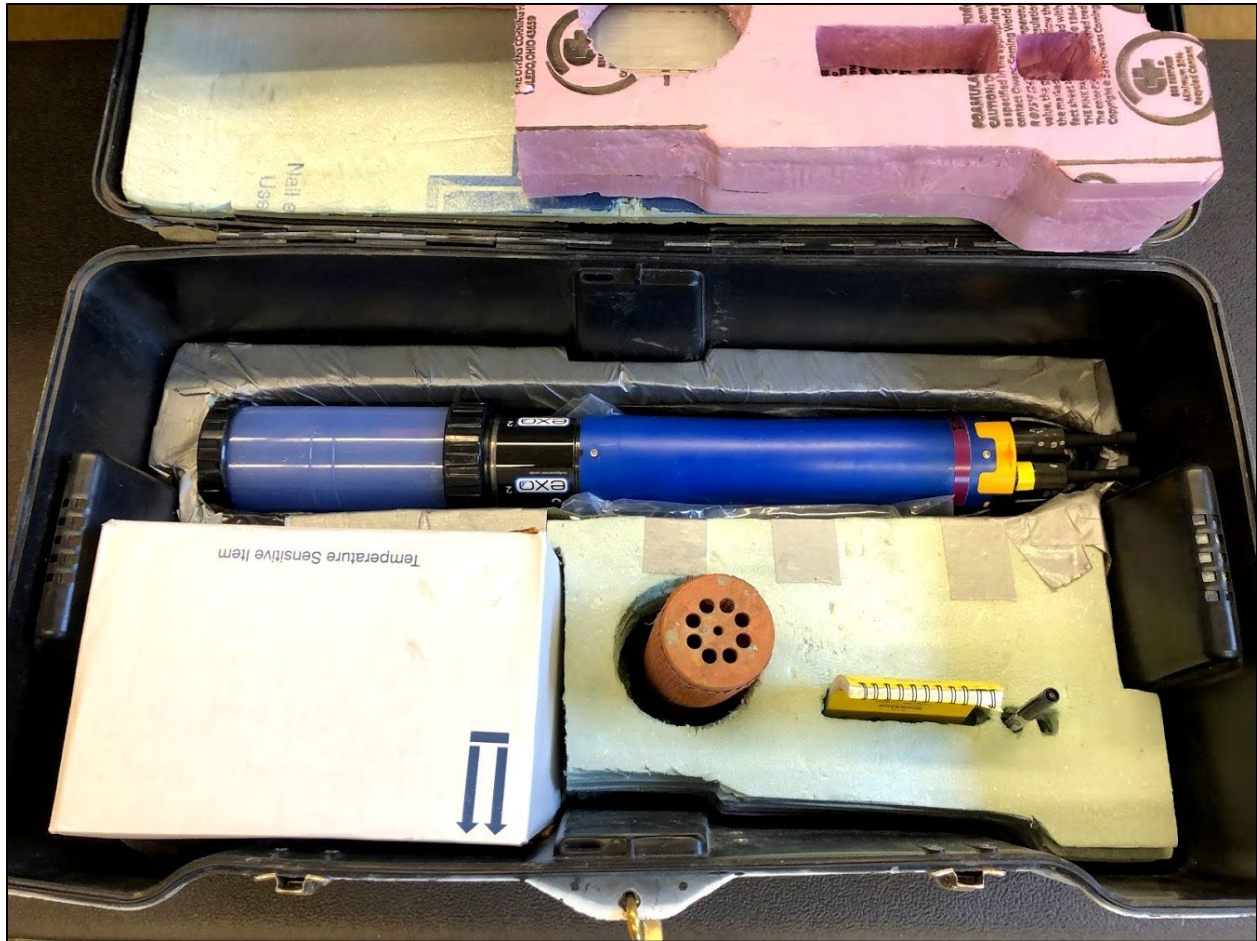
Figure 2. Layout of shipping container with sonde, copper guard, logbook, marker, and cooler. SOP's, datasheets, shipping labels, and zip-ties will accompany each shipment.
