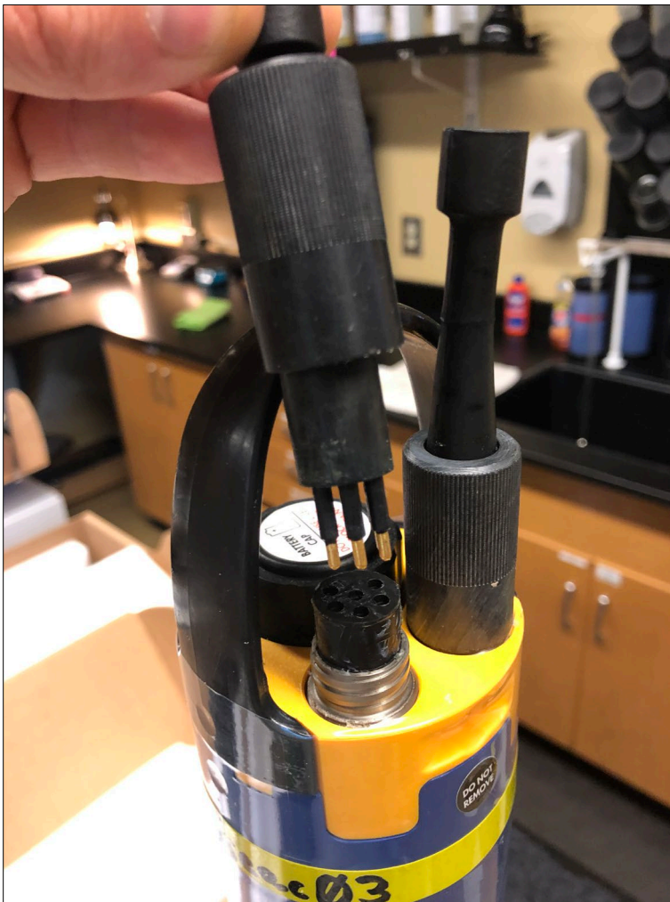
Figure 4. Dummy connectors being attached to the sonde.
