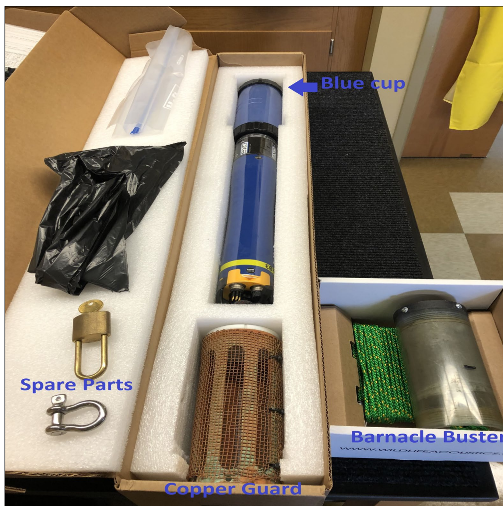
Figure 3. Layout of shipping container with sonde, spare parts, plastic bags, and instructions. The barnacle buster is included in a separate box.
