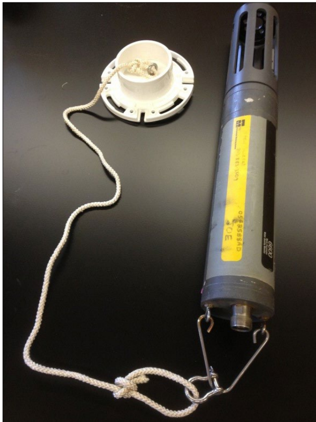
Figure 11. Example of sonde, shackle, rope, eye bolt and flanged cap.
