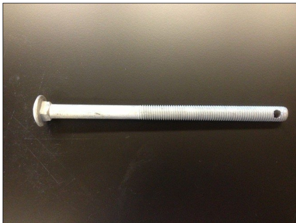
Figure 10. Example of bolt with hole drilled into it to accept lock.
