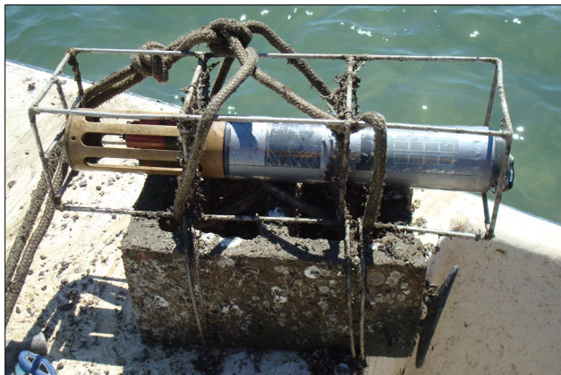
Figure 3. Sonde mounted inside of a modified crab pot at site CALOmidm02.
