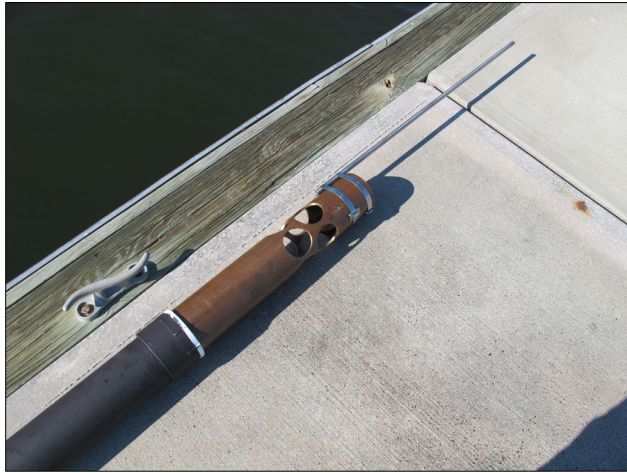
Figure 13. Sonde housing with brass end and anchor stake.
