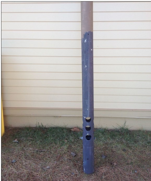
Figure 7. PVC pipe with flow holes and bottom bolt.
