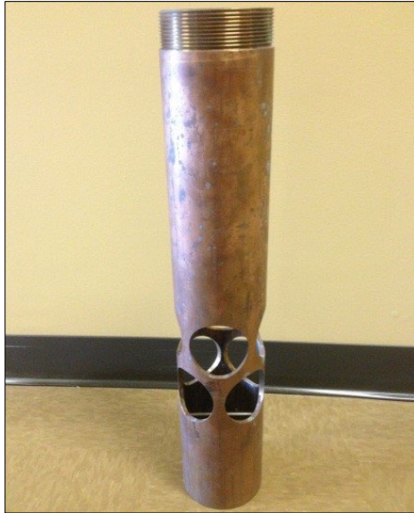
Figure 2. Two-foot schedule 40, 4-inch (10.16 cm), brass terminal end.
