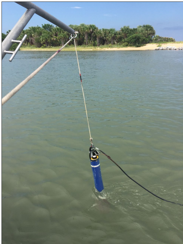
Figure 5. Sonde being lowered into the water to complete the hydrographic profile.
