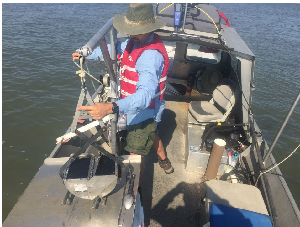
Figure A-6. Retrieval of the Ponar sampler and placement on the sample processing table.
