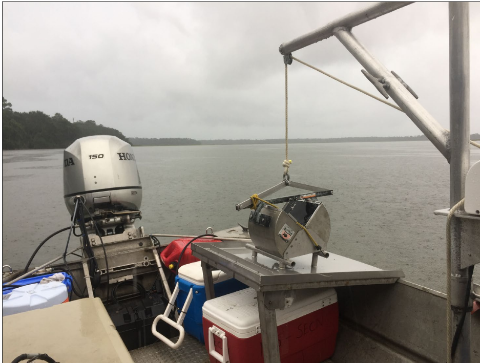
Figure A-1. General setup of boat, sample processing table, Ponar sampler, winch, and coolers.
