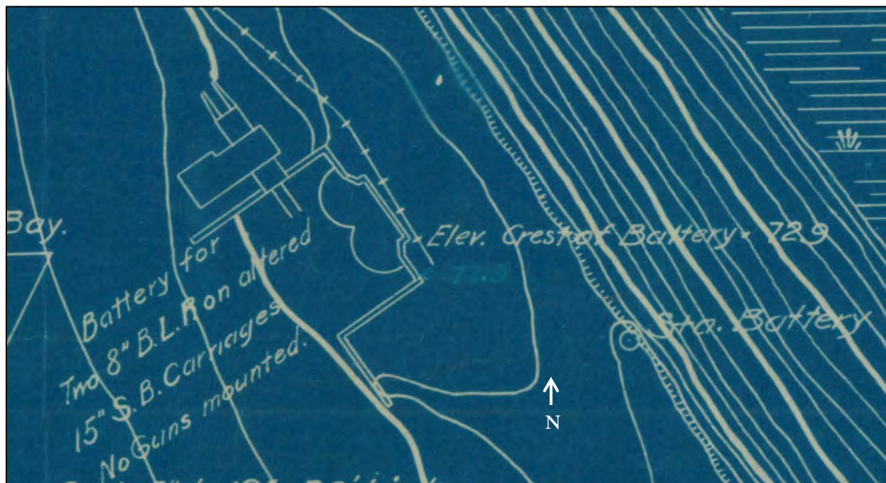
FIGURE 14. Layout of Spanish-American War Battery and bombproof magazine in December 1899. (Source: Benyaard, 1899 [March])
