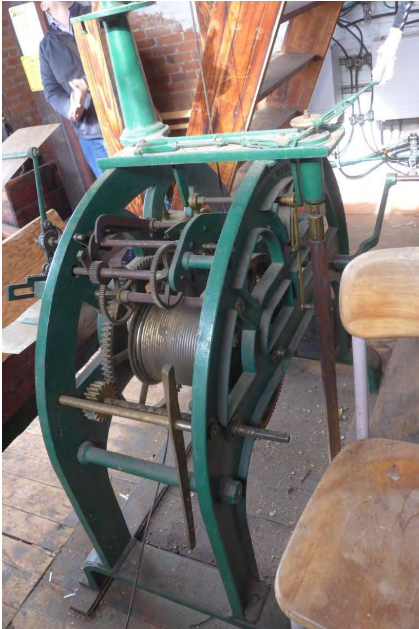
Cumberland Town Hall – Interior – Historic Finishes and Elements Tower – Fifth Floor Original Clock Mechanism
