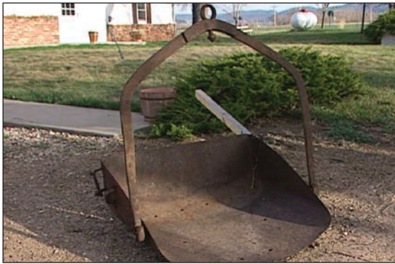
Horse or mule-drawn shovels, called slip-arounds or fresnos, cut the ditches.
