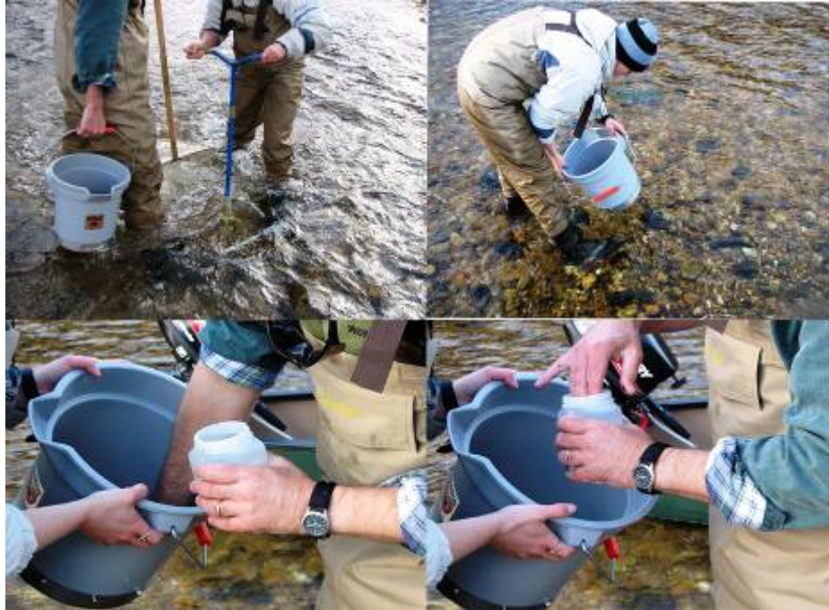
Figure 2. Placement of sampling net on stream bottom and agitation of substrate with garden tool (top left), washing the fine sediments from the sample using the wash bucket (top right), and transferring sample from wash bucket to sample container (bottom). Note that sample container is always held over wash bucket to ensure that sample is not accidentally spilled.
