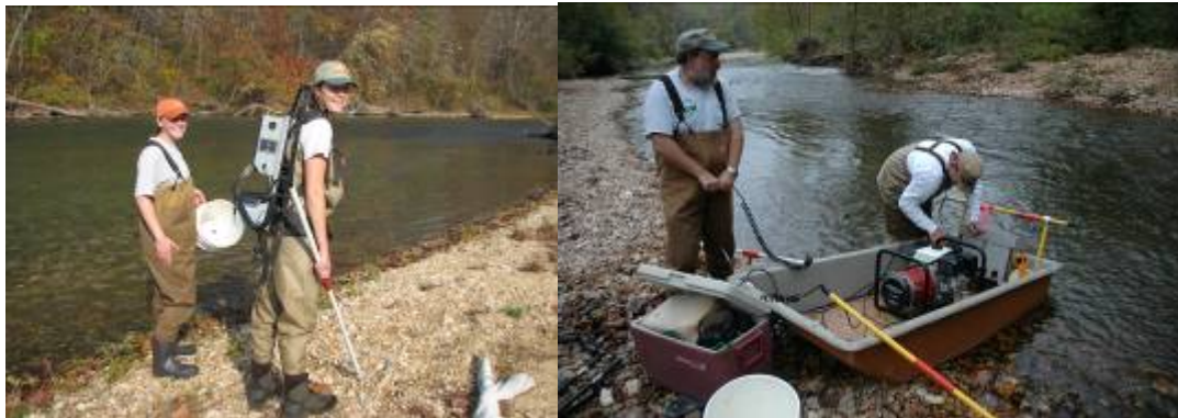
Figure 1. Backpack (left) and towed barge (right) electrofishing gear used in wadeable spring-runs.
