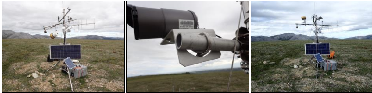
Figure 17. Mt. Noak climate station, July 27, 2017. Pre-visit station damage is shown (left). A new phenology camera was installed at the site (middle). Photo after maintenance (right).
