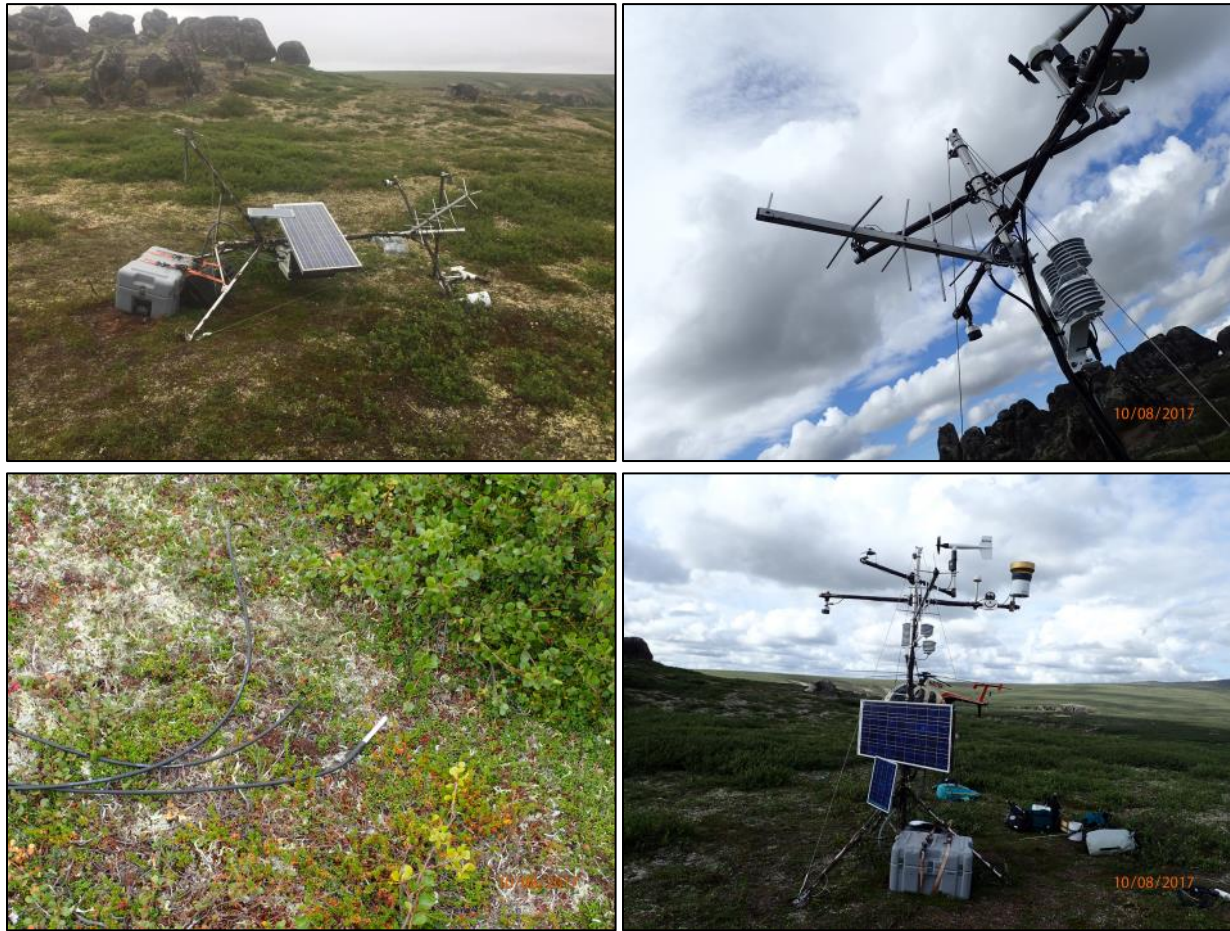
Figure 22. Serpentine climate station on July 3, 2017 (upper left; photo Matt Nolan) and August 10, 2017. The upper right photo shows the station before repairs, the lower left photo shows the soil temperature sensors as found before reinstallation on August 10. The bottom right photo shows the station after repairs and annual maintenance.
