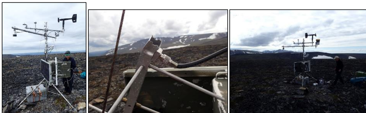
Figure 20. Ella Creek climate station July 24, 2018 before (left, middle) and after (right) station maintenance.
