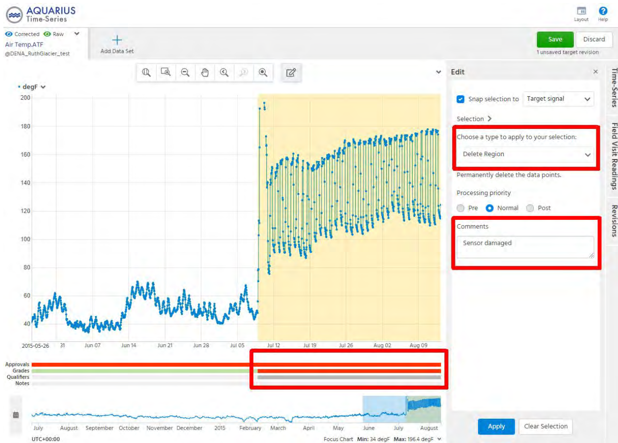
Figure SOP 11-22. An example of data retrieved from a damaged air temperature sensor. Erroneous measurements on June 8. The “Delete Region” correction action deleted all values during the selected time period. A custom comment (“Sensor damaged”) was added to describe the delete region action. For damaged sensors, the quality grade for the time period should also be set to “-2- Unusable” with a descriptive note added to describe the reason for grading.
