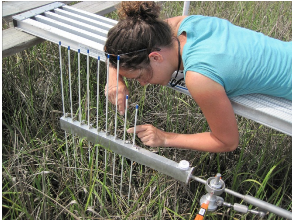
Figure 10. RSET with fiberglass pins being lowered to the ground surface. Place the clip back on the pin and repeat this for the other eight pins.
