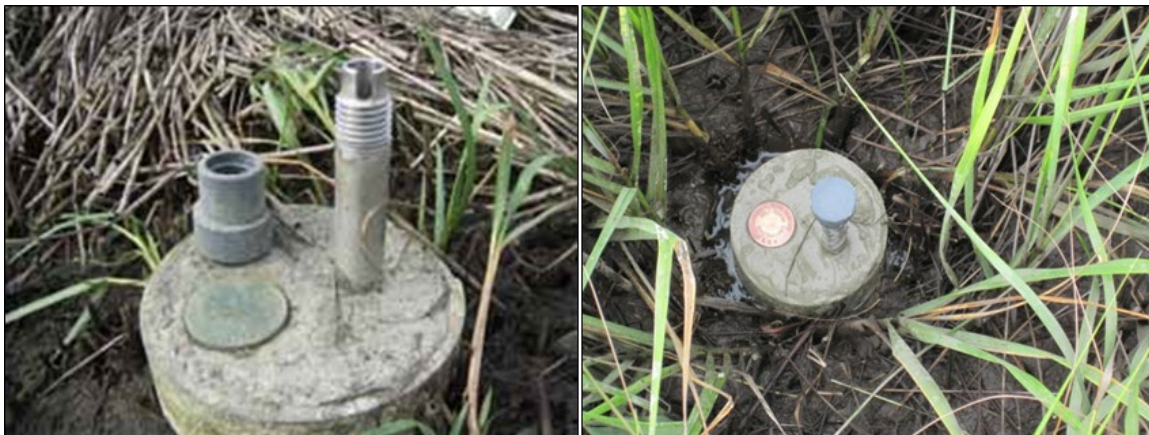
Figure 4. Deep rod benchmark / monument and receiver capped (right) and receiver uncapped (left; from “Taking Your SET Readings” in Cahoon and Lynch 2003).
