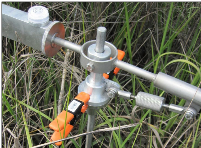
Figure 9. Clamp RSET to collar using spring clamps.
