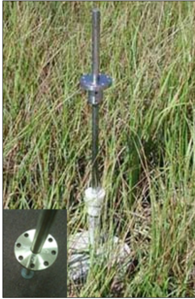
Figure 7. RSET insert collar mounted to receiver. Inset: close-up of insert collar (modified from “Taking Your SET Readings” in Cahoon and Lynch 2003).
