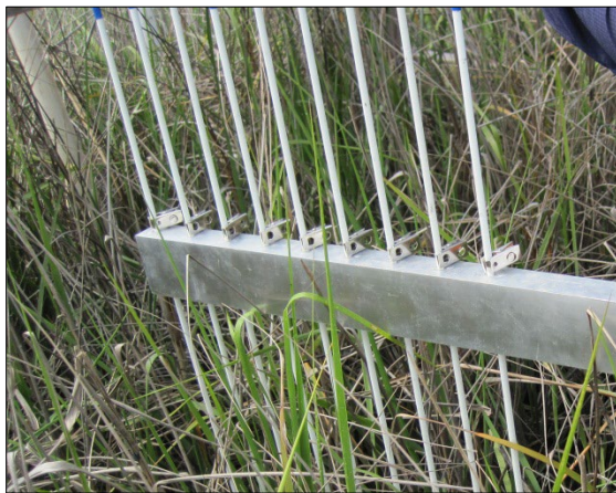
Figure 6. Fiberglass pins installed in the RSET with badge clips.
