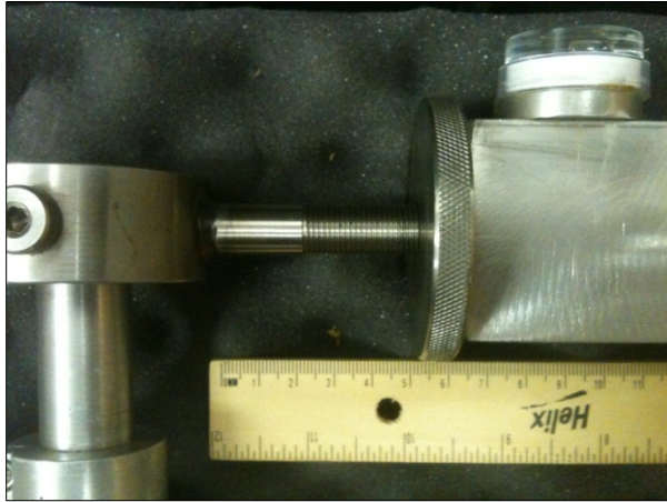
Figure 5. RSET arm locked into position 6 centimeters from the exterior edge of the pivot joint.
