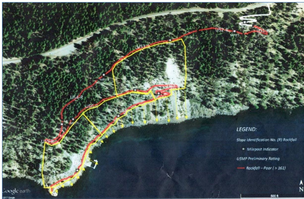
Figure 4. Planned rockfall mitigation and scaling areas on the Cleetwood Cove trail. Areas outlined in yellow indicate fall zones for scaled rock. Yellow arrows indicate pathways where the scaled rock and debris will fall. Map provided by the Federal Highways Administration.
