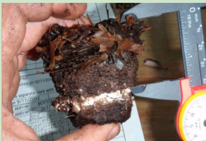
Figure 2. Measuring accretion, which is the material deposited above the white line. The white line is feldspar, a mark layer placed at the site on a previous sampling event. Here we can see turtle grass ( Thalassia testudinum ) that is becoming incorporated into the soil. This sample was taken at Biscayne National park.
