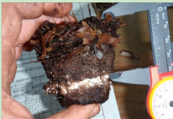
Figure 2. Measuring accretion, which is the material deposited above the white line. The white line is feldspar, a mark layer placed at the site on a previous sampling event. Here we can see turtle grass ( Thalassia testudinum ) that is becoming incorporated into the soil.
