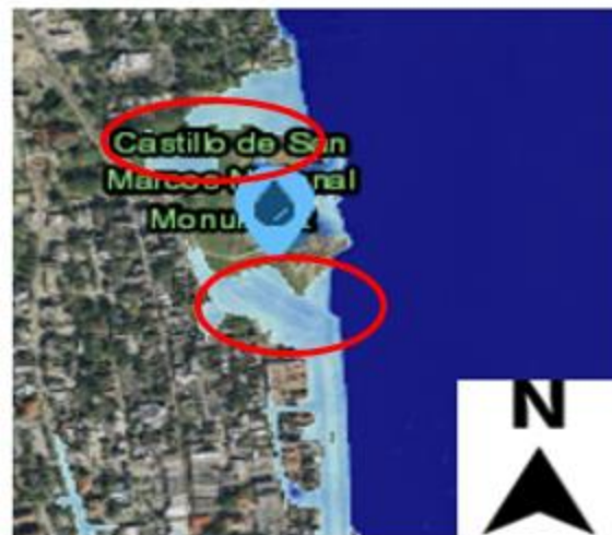
Figure 5: Aerial view of the potential flooding areas due to a storm surge of 3 feet above MHHW (NOAA Sea Rise Viewer tool).
