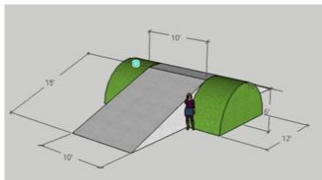
Figure 53: Side view of proposed ramp solution
