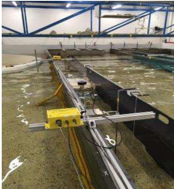
Figure 24: Wave Channel with Pier and Capacitance Wave Height Gages (MIDN Ian Myers, 2020)
