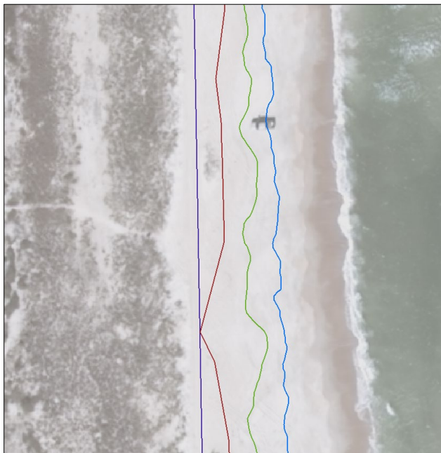
Figure 48. Screen capture of 'ArcGIS' map view displaying the edited high tide shapefile.
