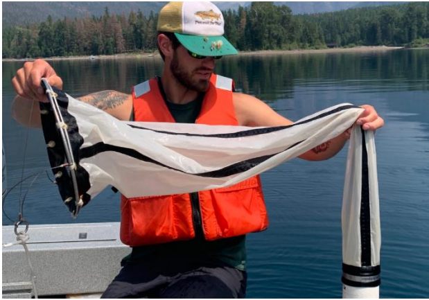
Figure 3. Retrieving the plankton net and decanting off much of the water to concentrate the sample.
