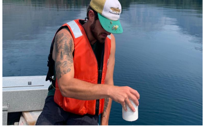
Figure 3. Retrieving the plankton net and decanting off much of the water to concentrate the sample.
