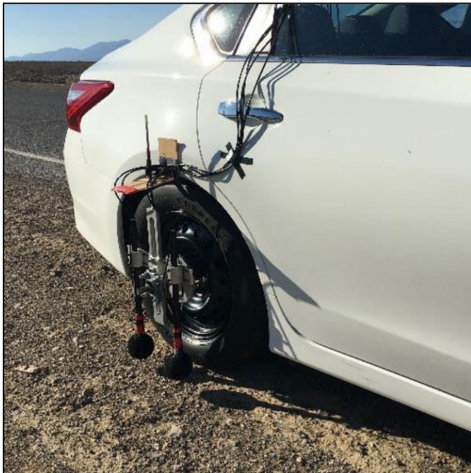
Figure 6. Example of OBSI microphone array mounted on a passenger car (VOLPE CENTER).
