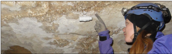
Data loggers record cave air temperature and relative humidity to help document the effects of global climate change on the abundance, occupancy, and habitat use of several monitored cave dwelling taxa including federally listed Indiana bats ( Myotis sodalis ), hibernating below. NPS photo / CUPN staff.
