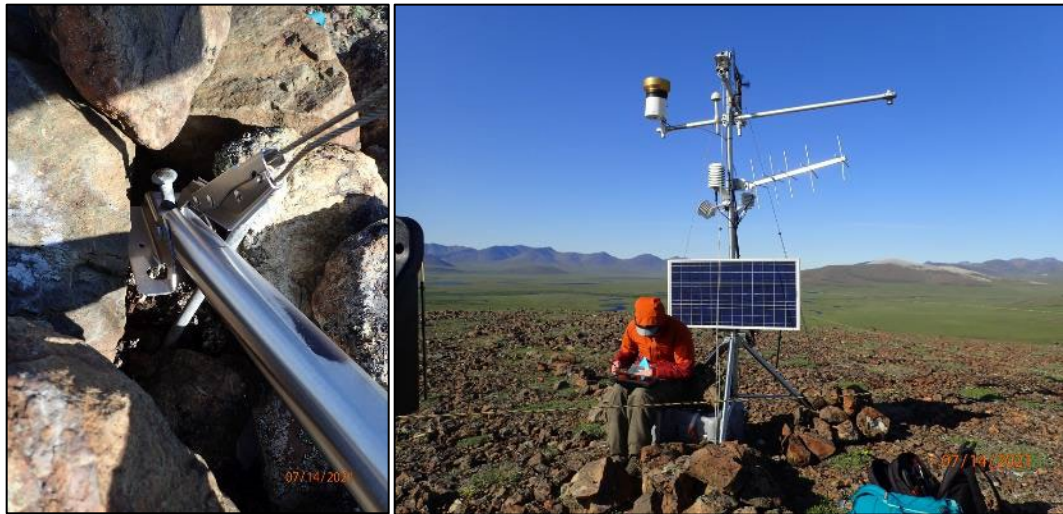
Figure 7. Howard Pass climate station, July 14, 2021. The NE tripod leg had been pulled out about four inches (left).
