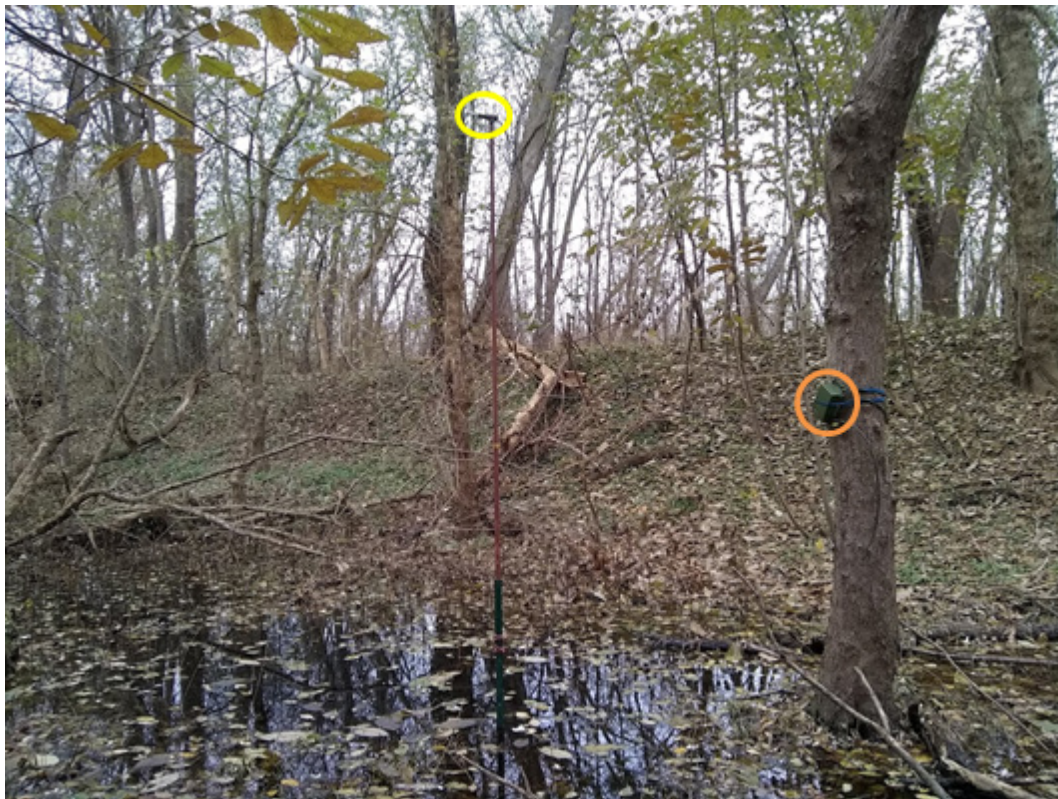
Figure 2. Typical passive acoustic detector attached to a tree (orange circle) with microphone (yellow circle) on the top of the corresponding pole in Chesapeake and Ohio Canal National Historical Park (NPS/SABRINA DEELEY)
