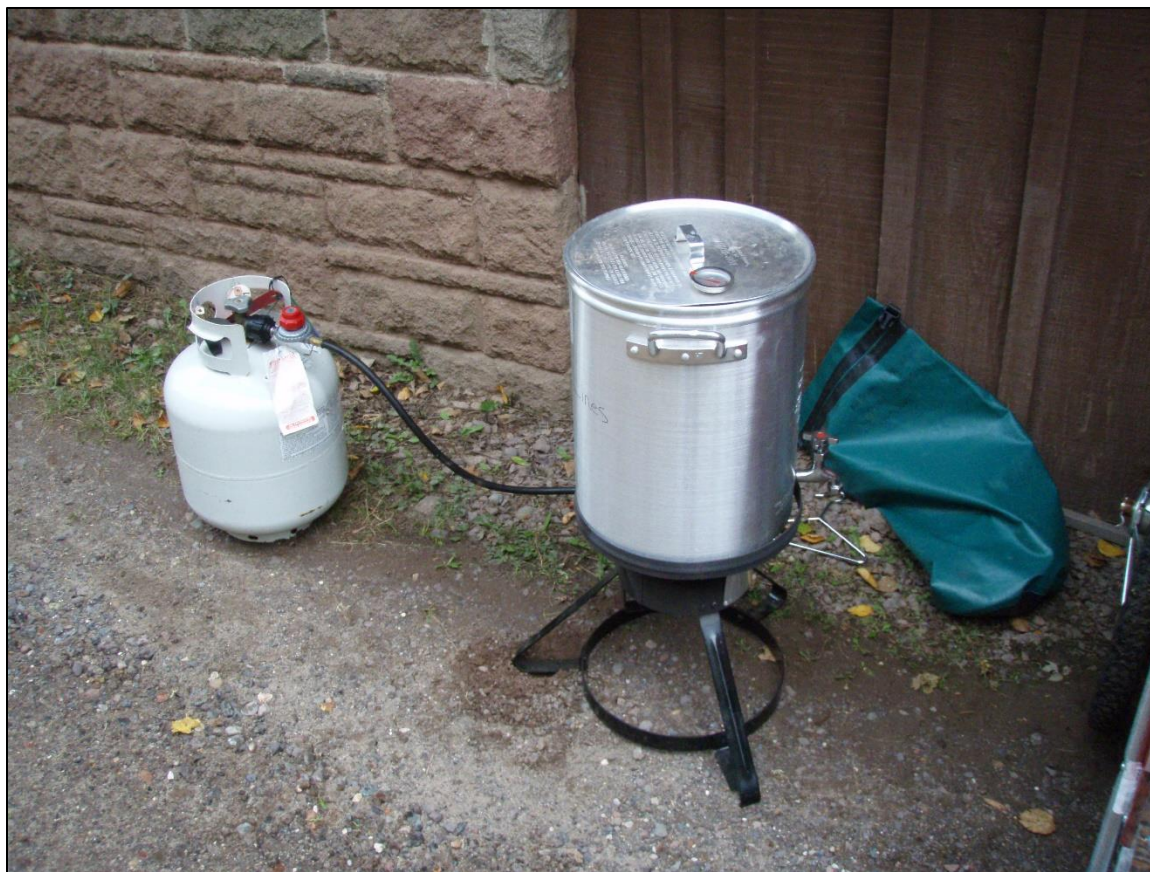
Figure 1. An example of a propane burner and pot used to heat water to 140° F (60° C) for decontaminating non-electronic equipment. Any large pot and heat source is acceptable, however a thermometer should be used to verify that sufficient temperatures have been achieved.
