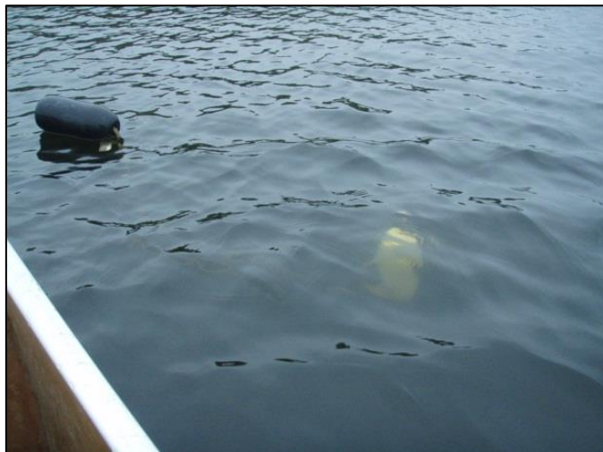
Figure 23. The surface and sub-surface buoys following deployment on a non-motorized lake. The sub-surface buoy is about a meter below the surface.
