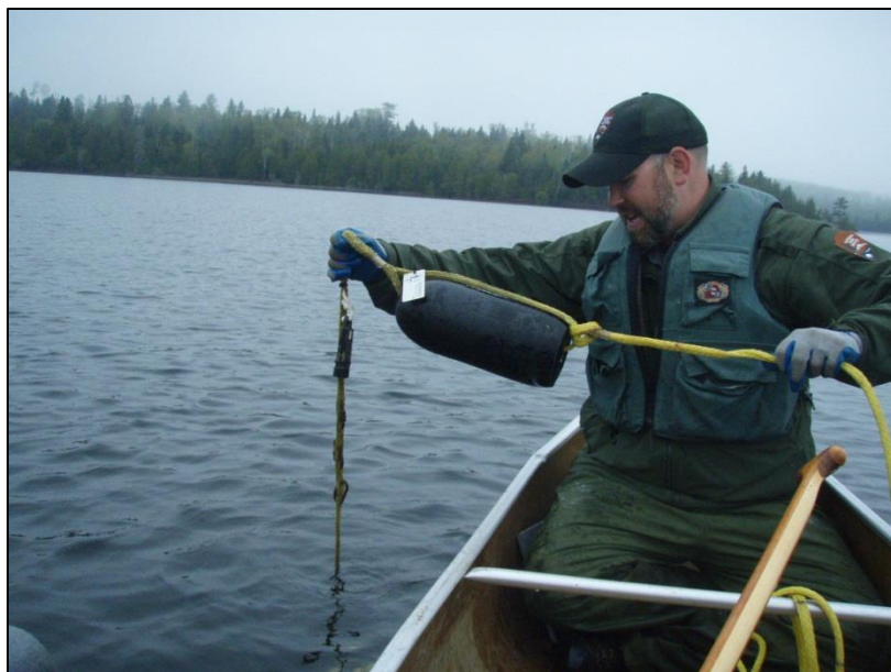
Figure 21. Instrument line deployment 2. About 1 m is the ideal amount of slack between the surface (black) buoy and the sub-surface buoy (under the water, with anchor resting on the bottom). The line between the buoys should be about 2.5 m long, for a sub-surface buoy that is to be deployed 1.5 m under the water. The yellow line attached to the right side of the black buoy is an extra length (about 3 m) of line attached to the surface buoy for easy retrieval, just in case the instrument line was too short and sunk the surface buoy.
