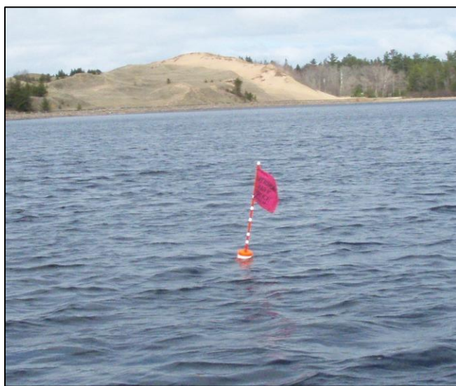
Figure 15. Example of a high-visibility staff buoy that can be used in areas with motorboat traffic. The buoy in the picture was deployed as part of the array at Grand Sable Lake, Pictured Rocks National Lakeshore.
