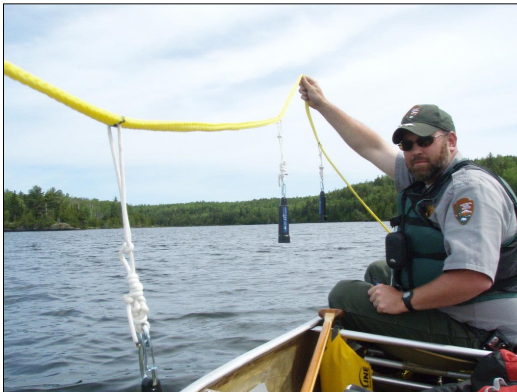
Figure 3. An array being deployed at Lake Richie, Isle Royale National Park. Sensors are clearly visible and are spaced 1 m apart (NPS-GLKN photo).
