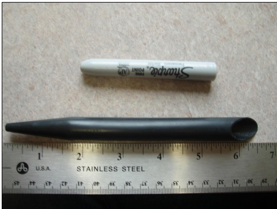
Figure 12. A 1/2-inch fid used for splicing 3/4-inch braided polypropylene line. If you don't have a fid, you can make one for 1/2-inch line using the tube from a Sharpie marker.
