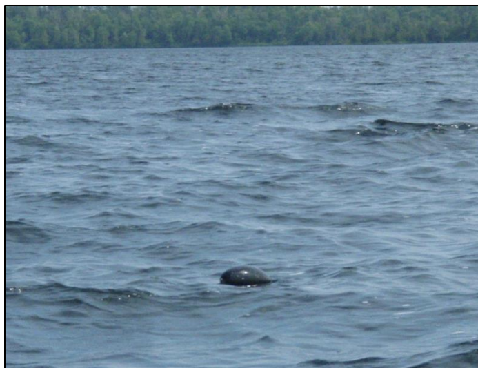
Figure 14. Example of black array buoy meant to help the buoy visually blend with its surroundings when on a lake in designated wilderness. Siskiwit Lake, Isle Royale National Park.
