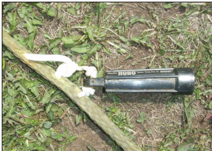
Figure 17. Parachute cord is used to attach a temperature logger to an instrument line. The end of the line is tucked into the hollow core instrument line (upper left), while a zip tie was affixed around the line to hold the end in place (not shown).
