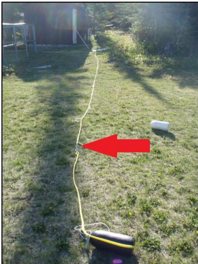
Figure 18. An array being assembled on land. The buoys are in the foreground and the anchor bags and grab line in the background. Please note, the subsurface buoy has not been attached yet, nor have the loggers. The subsurface buoy will be attached near the swivels and quick links in the foreground (indicated by red arrow).
