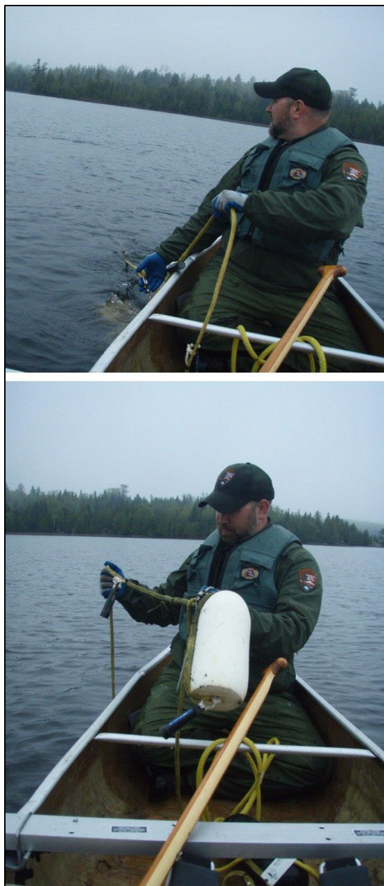
Figure 20. Instrument line deployment 1. ( Top ) The grab line has been deployed (trailing off to the upper left underwater) and the instrument line anchor is about to be released. The instrument line and buoy are coiled forward of the canoe thwart. ( Bottom ) The line is being lowered slowly, and care is being taken to not hit the loggers on the side of the boat. The instrument line anchor is about 2 m off the bottom in this photo. The white buoy is the sub-surface buoy.
