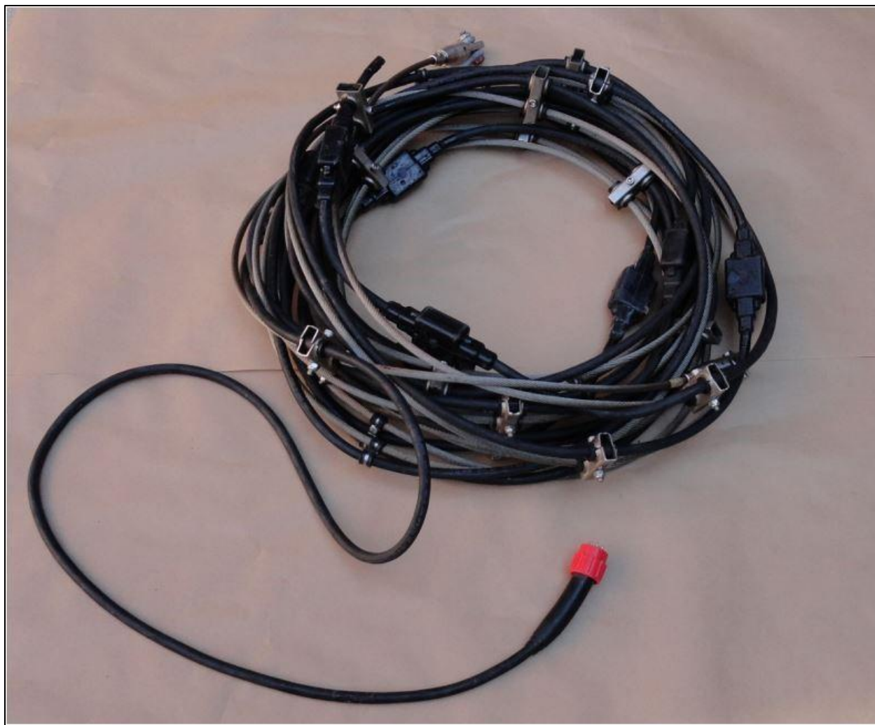
Figure 2. Thermistor chain to be deployed under an automated profiling buoy system (photo from University of Michigan Ocean Engineering Laboratory).
