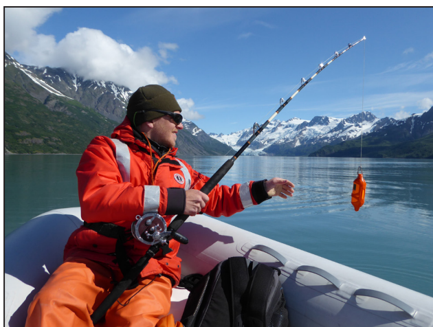
A researcher uses a fishing rod to deploy a CTD unit in McCarty Fjord. NPS Photo/D. Kurtz
